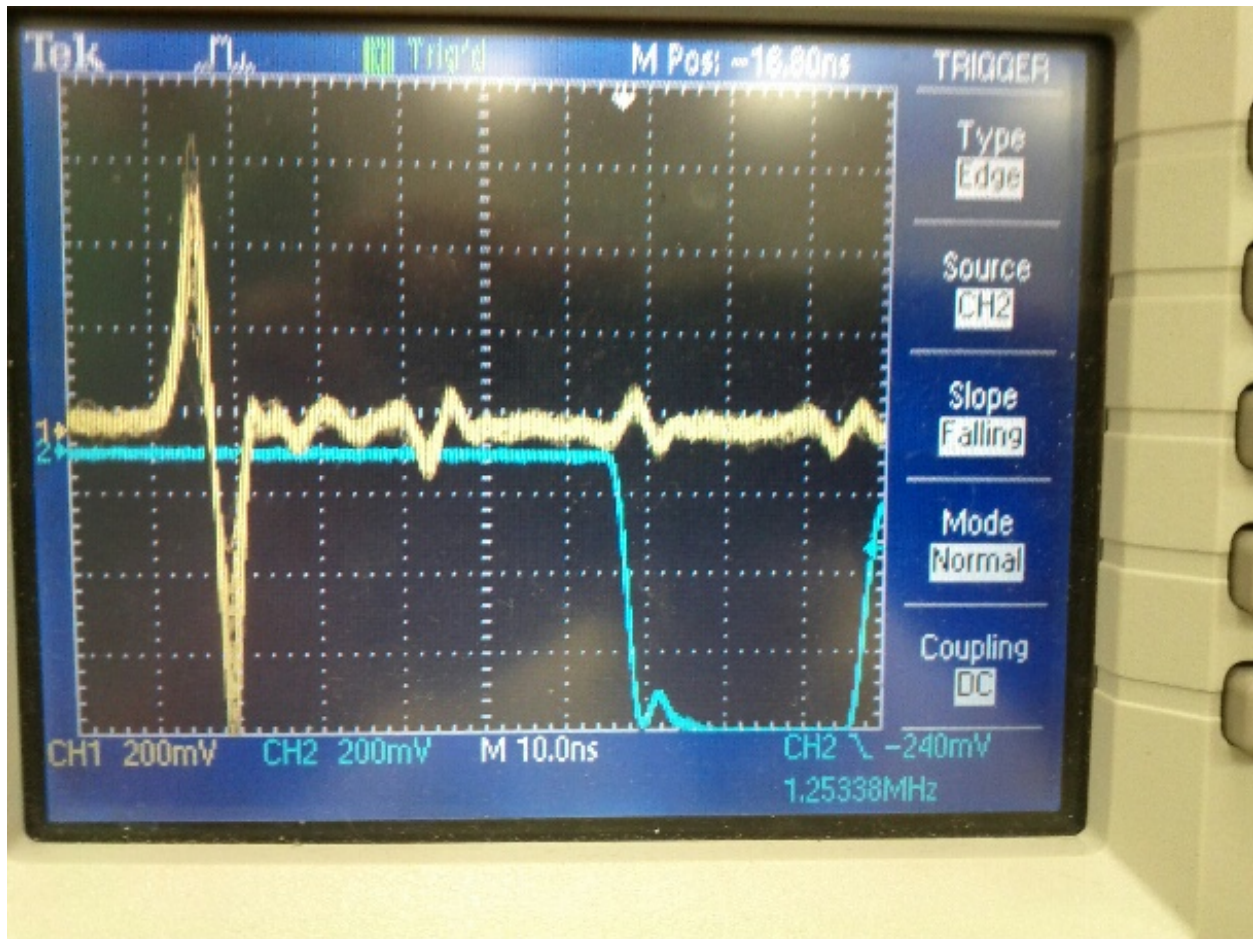
Figure 3.13: An oscilloscope trace (yellow) of the pickoff signal from a pulsed ^3\text{He} beam on the 70-degree line at TUNL. Amplifier noise is apparent at times beyond the signal. The blue trace is the logic timing pulse corresponding to the zero-crossing of the pickoff signal; it is used to stop the TDC. For this experiment, the beam was pulsed at 1.25 MHz.
