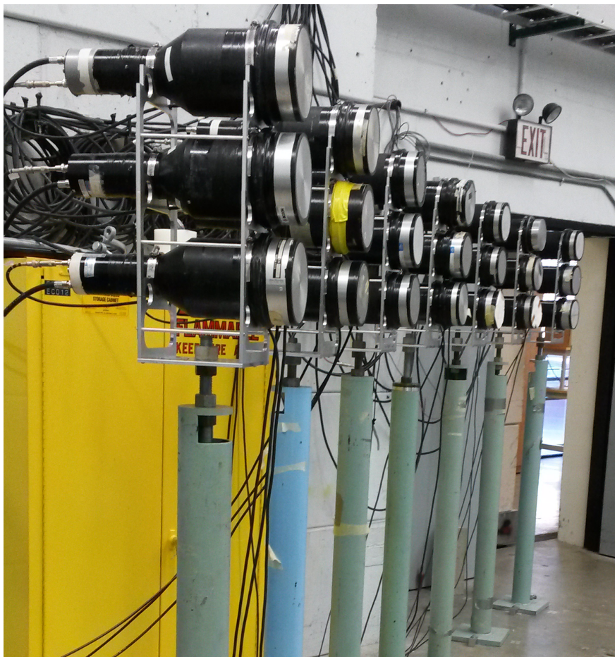
Figure 3.18: A photograph of the liquid-scintillator neutron detector array. 21 detectors were positioned between between 0^\circ and 18^\circ in 3^\circ increments. Three detectors were placed at each angle to increase the solid angle coverage. The middle detectors are placed at beam height, approximately 69.5" from the floor.
