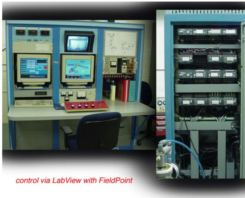
Figure 3-12: LabVIEW control system
