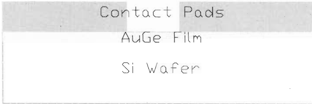
Figure 2.7: Cross section of Au_xGe_{(1-x)} thin film thermistor.
