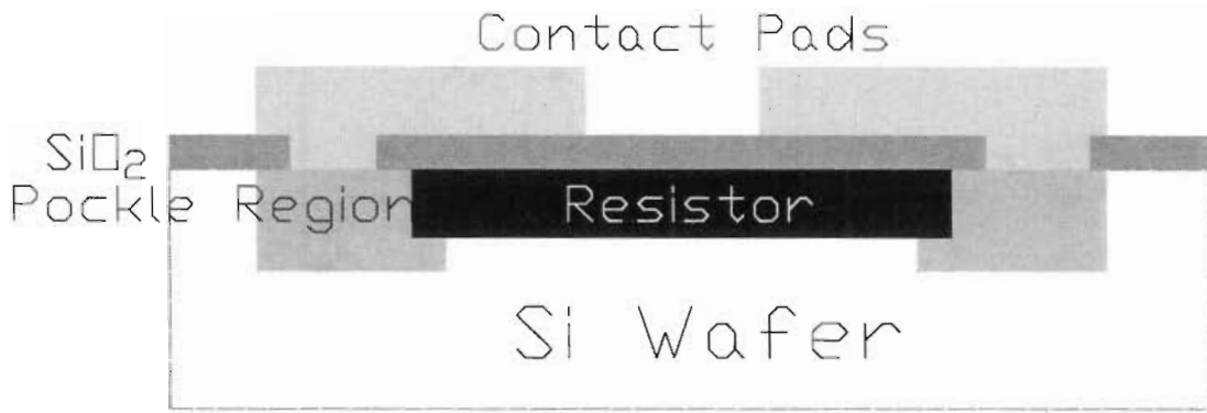
Figure 2.1: Cross section of P:Si thermistor after all production stages.
