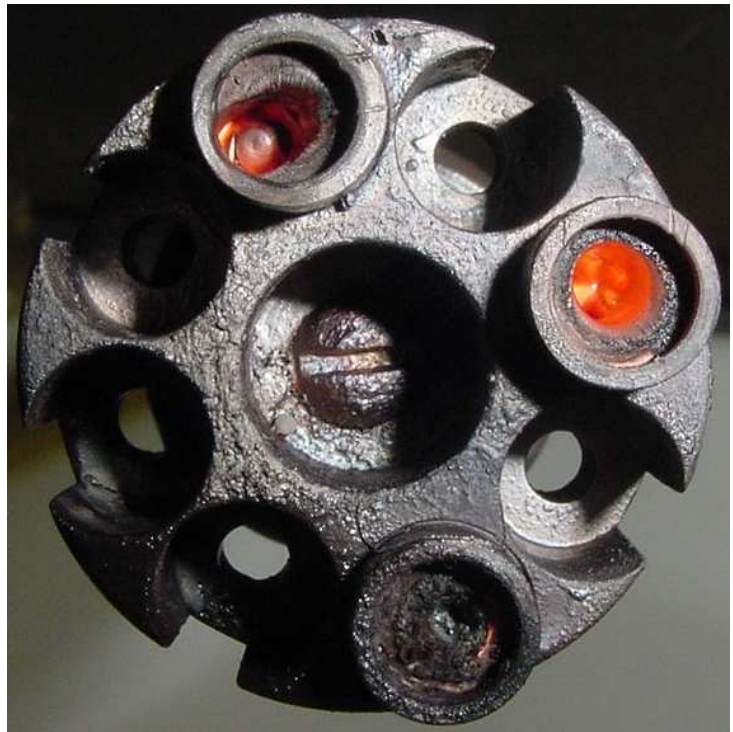
Figure 2.11: Scale cross-sectional view of a {}^7\text{Be} cathode (left). The Cu mold (brown) and Ag+Be matrix (grey) are shown. The bottom hole is for mounting in the target wheel. Photograph of the sputtered cathodes (right). The top left position held a {}^7\text{Be} cathode (see text).
