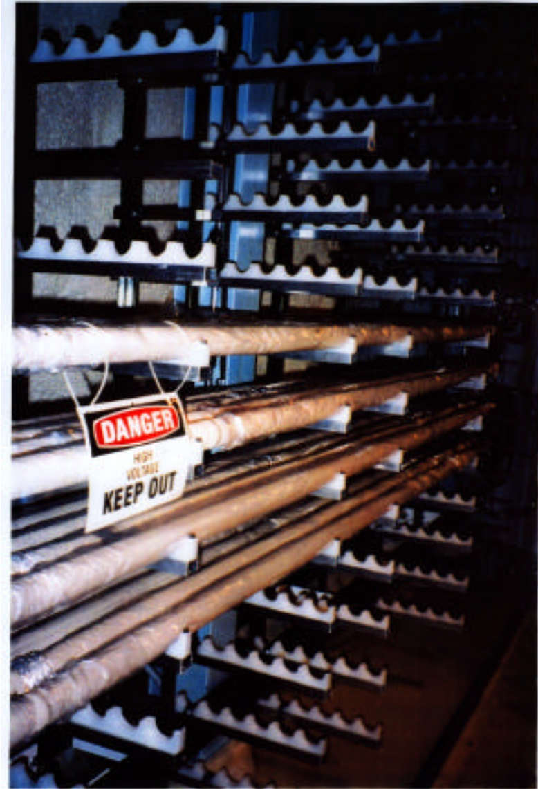
Figure 4.10: Underground NCD cool-down storage rack designed and built by the LBNL NCD collaborators. The counters shown have been temporarily assembled to be operated as strings ranging in length from 4 to 11 meters.
