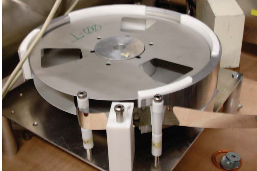
FIGURE 2.6: Prototype tape reel system. The tape reel rested on a motor-controlled reel table. A reel protector contained the tape during unexpected tension loss or motor runaway.
